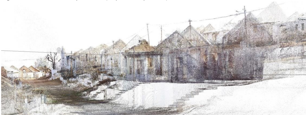
Fig 9 Point cloud survey - terrestrial (Cape Survey, 2019)
