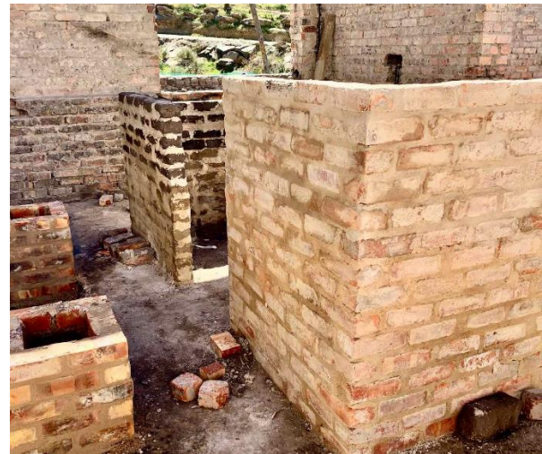
Figure 8: Trial panels using lime/sand mixes for plastering and laying brickwork. Left: Two separate lime plaster panels experimenting with water proportions. The shrinkage cracks in the lower panel show that too much water was added. Right: Trial samples of brick walls constructed using exclusively lime/sand mortars to convince an initially sceptical contractor that such lime mortars without Portland cement would be structurally sound. The wall in the foreground is constructed using modern fired bricks. The darker wall in the background experiments with bricks recovered from the fire damaged ruins. (Image ARCON, 30 August 2019)
