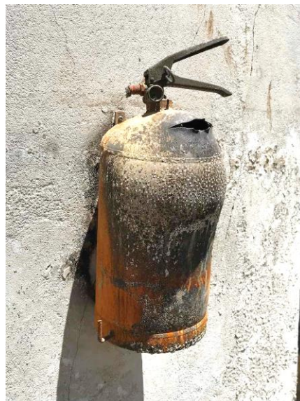
Right: The fire spread so rapidly that the fire extinguishers could not be used. This example was left to explode on its wall bracket. (Image: ARCON, 24 January 2019)
